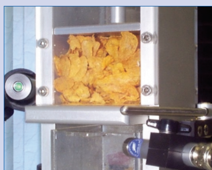
Figure 1. The Video Playback Indicator is set up in the frame view of the test sample on the TA.XT plus Texture Analyser,
